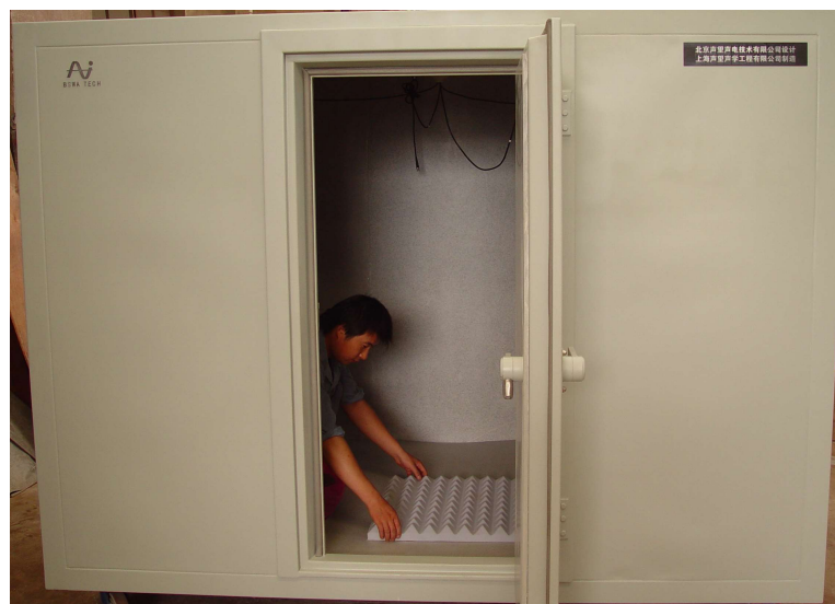
Figure 1- R-Cabin designed and built according to SAE J2883.
